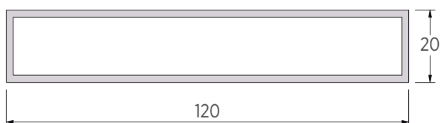
PROFILATO - gr. 1469 al metro lineare PROFILE - gr. 1469 for linear meter
